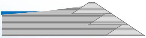
**Downstream tailings dams, with tailings discharged towards them, lead to super-elevated tailings, which are susceptible to liquefaction**
