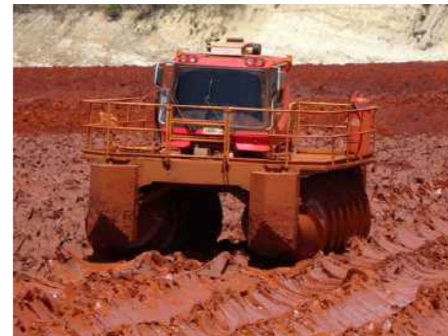
Figure 5. Amphirol or scroller on red mud
