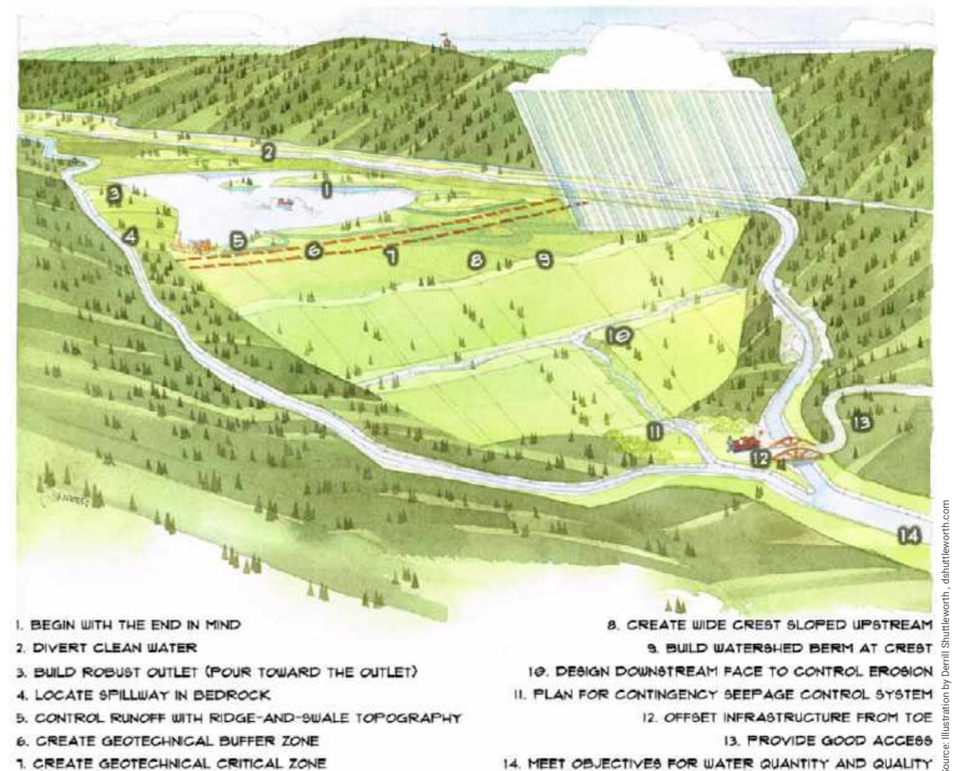
Figure 4. Good practices for design of tailings landforms
