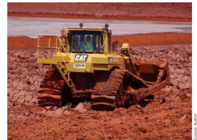
Figure 6. D6 Swamp Dozer on red mud
