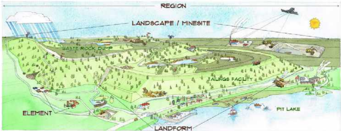
Figure 1. Four scales of landform design
