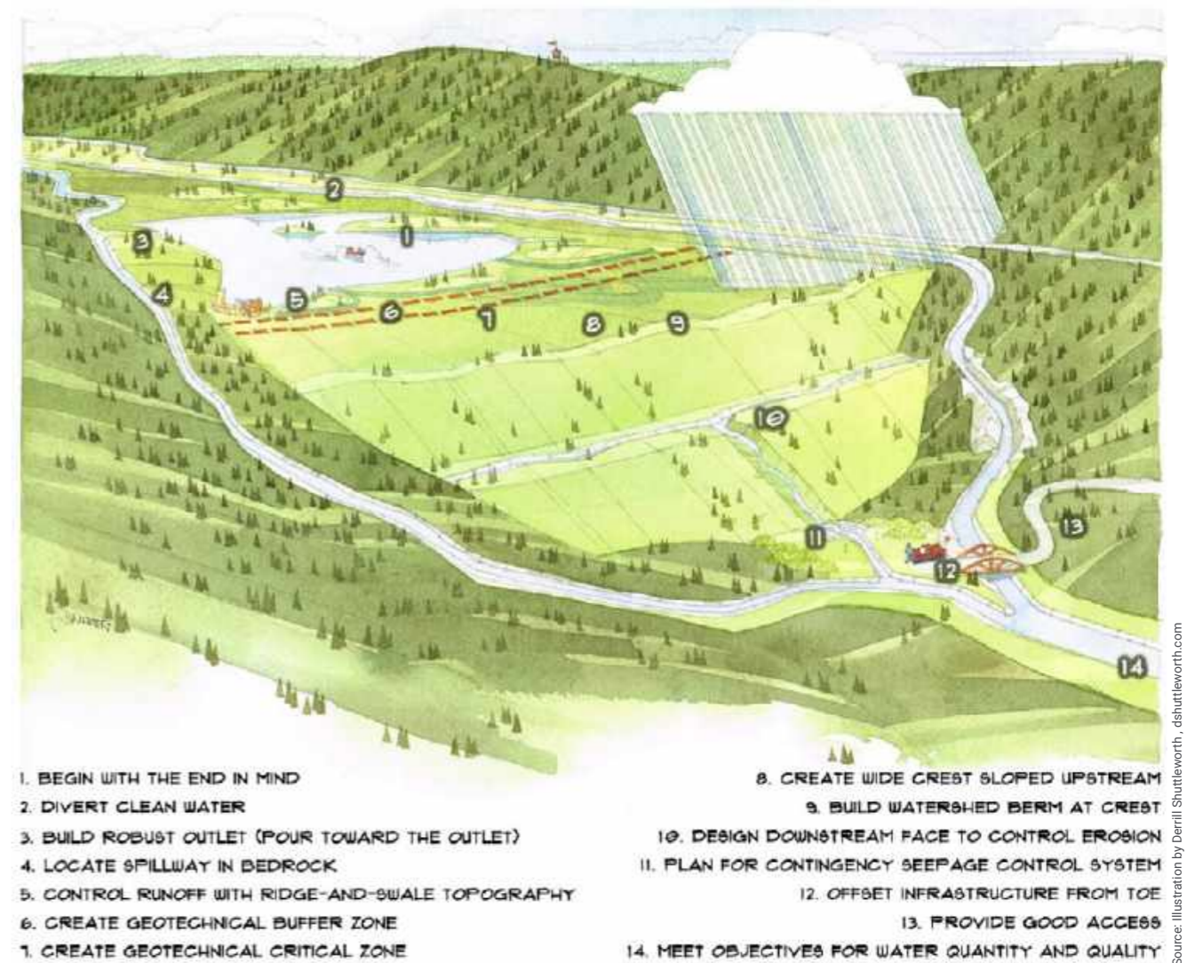
Figure 4. Good practices for design of tailings landforms
