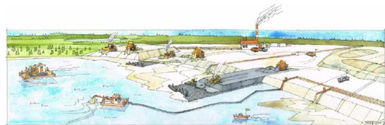
Figure 5. Common methods for capping soft tailings (McKenna et al. 2018)
