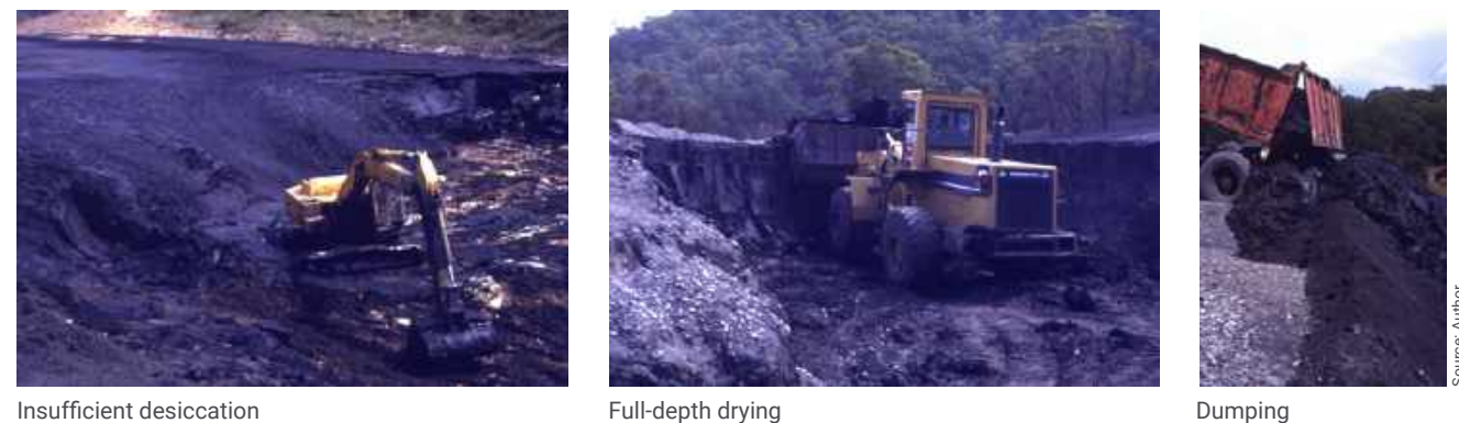
Figure 4. On-off coal tailings cells, employing solar and wind drying, harvesting and disposal with coarse reject
